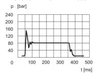
Diagram noted passing from maximum flow rate to zero flow rate and vice versa
